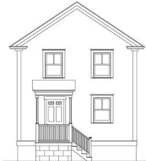
▲ Inappropriate Cinderblock porch base.
