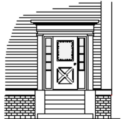
▲ Inappropriate Door design and aluminum screen.
