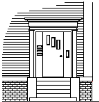
▲ Inappropriate Sidelights replaced by mailboxes and buzzers.
