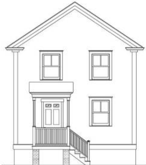
▲ Inappropriate Brick or wood columns without infill.
